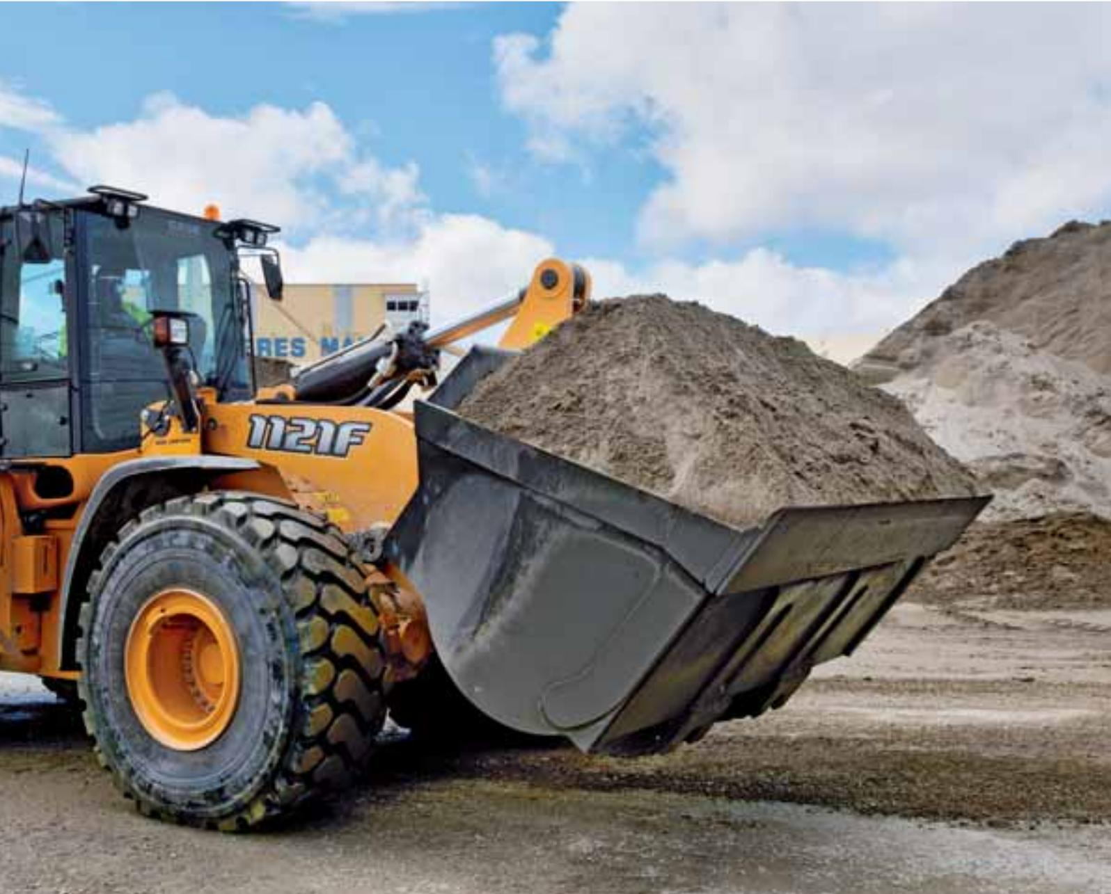
**2011** *The first wheel loaders with SCR engine technology and Proshift transmission lead to faster cycles and fuel economy.*
