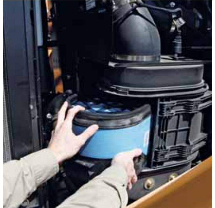
The air filter is easy to remove and the dust is aspirated and ejected in the exhaust
